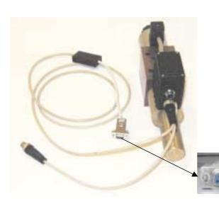
A special cable provides the valve connection with the computer via a 5-pole connector M12 x 1 (male plug), the connection with the supply voltage via a 5-pole connector M12 x 1 (female plug) and the connection with the series port of the computer via a 9-pole connector CANNON 9. A part of the connection cable is also build up by an interface providing adaptation of the signal voltages.
